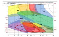
The crossover chart describes where your sails fit in terms of wind angle and wind speed. It takes time to make this chart accurate. We can make a generic one for any boat, yet each time spent on the water is valuable in perfecting this chart. An accurate chart minimizes decision making when making a sail call.
