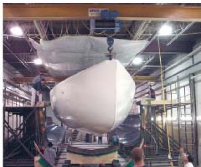
Hull number one gets hoisted from the mould
